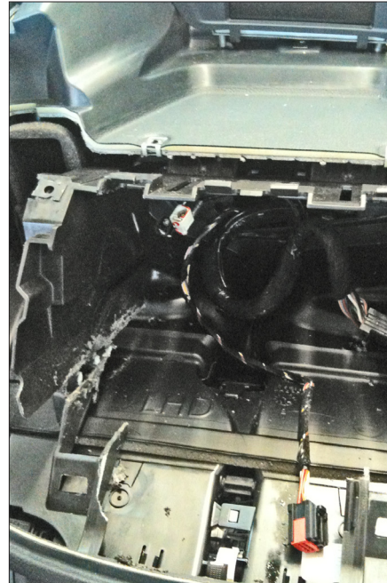
17. Dashboard after plastic cut out
